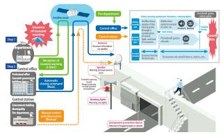
Automatic closing system mechanism
